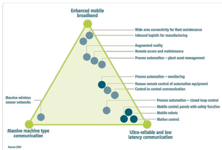
Figure 3: Selected manufacturing use cases and their positioning on the 5G services triangle [4][5].
