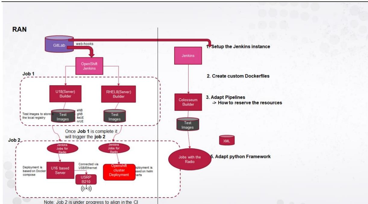
Figure 1: COLOSSEUM extension to OAI automatic testing framework
