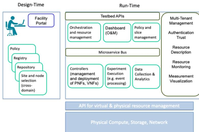
Figure 4: Software architecture and tools for experiment design and run-time
