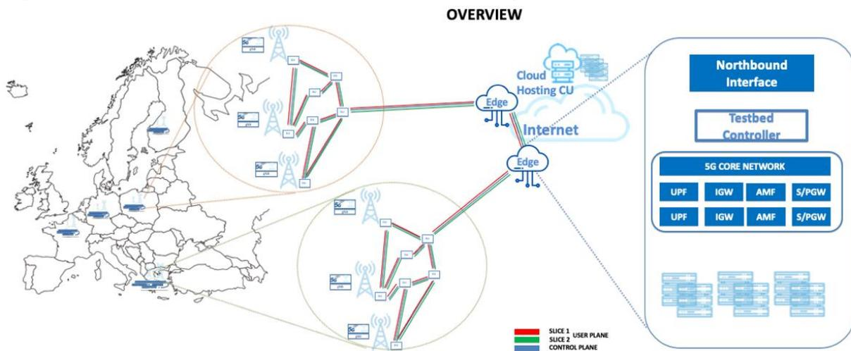
Figure 6: A use case that considers deployment of a 5G network spanning the entire continent
